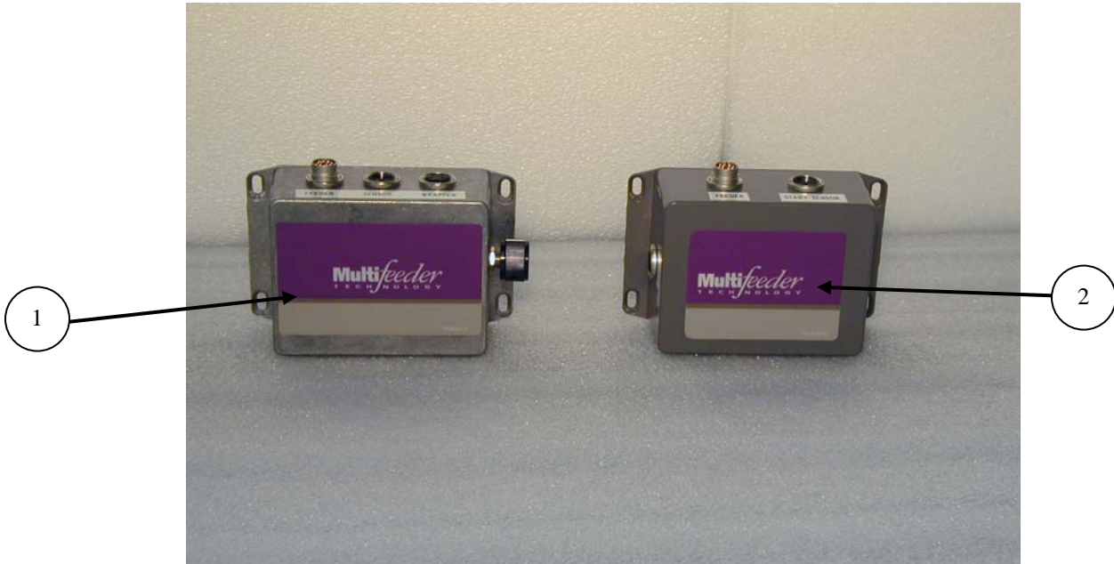
Figure 12.1 – IP Feeder Interface Boxes
