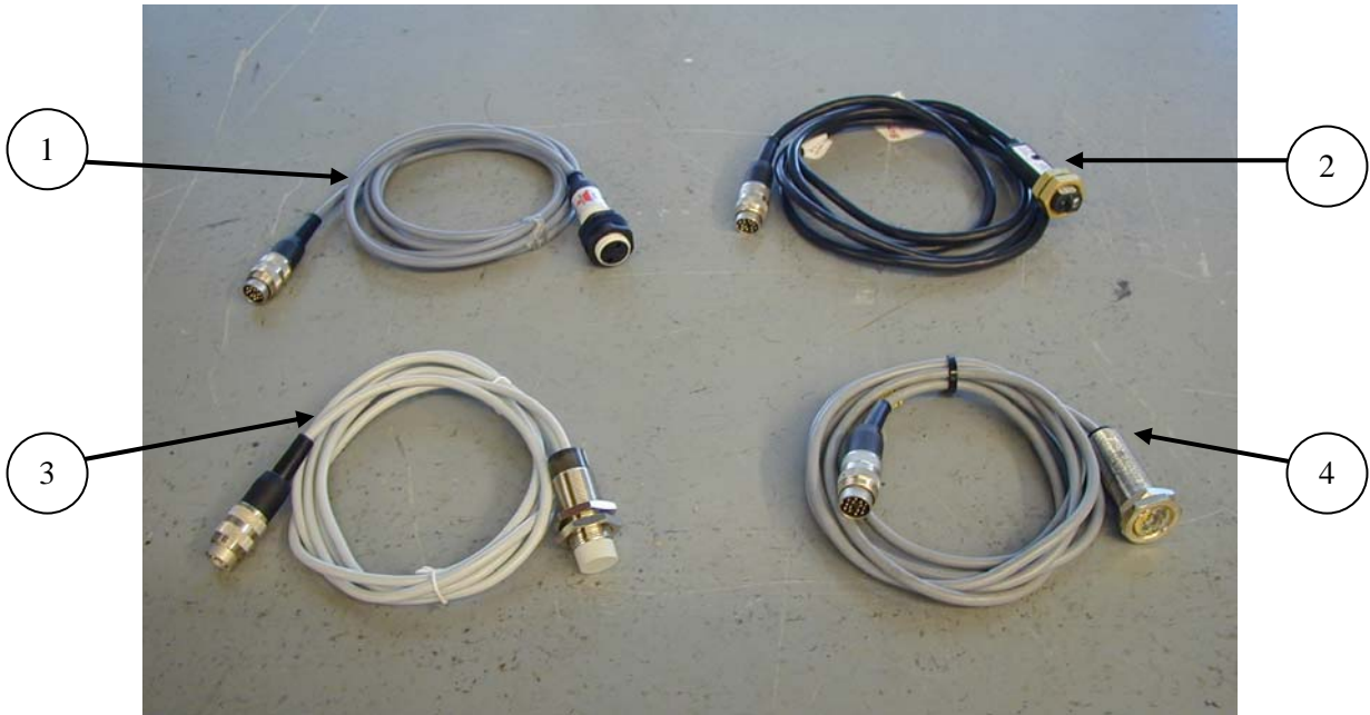
Figure 9.1 – IP Feeder Start Sensors
